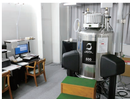
NMR (JNM-ECZ500R) Structural analyzer based on nuclear magnetic resonance to investigate the molecular structure, intermolecular interactions, and molecular motion of various kinds of molecules.
